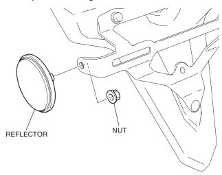
4. Install the reflector stay as shown.
