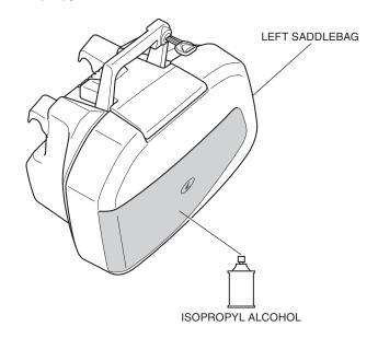
3. Peel off the adhesive backings on the left saddlebag cover as shown.
